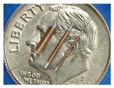
*Electromagnetic sensor micro-coils on a dime for scale* [*Illustration courtesy of Intricon*]
