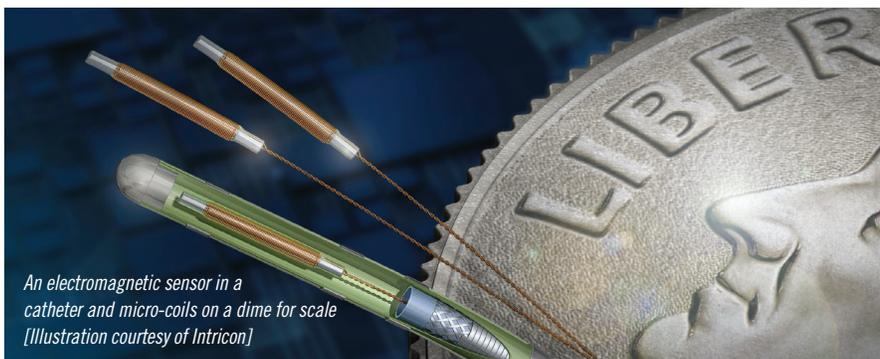
*An electromagnetic sensor in a catheter and micro-coils on a dime for scale
