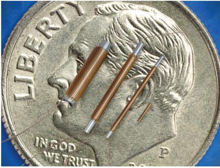
Electromagnetic sensor micro-coils on a dime for scale
